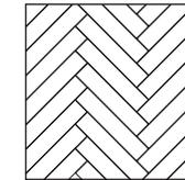
**ALL LAMINATE HERRINGBONE JOINTS MUST BE GLUED WITH PVA GLUE**
